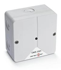
Intelligent Input/Output module for the Loop 3000 for the control of external optical and acoustic signaling devices with bidirectional isolator according to EN 54-17 and EN 54-18. Including one monitored fault input and one potential free relay output for signaling devices.
